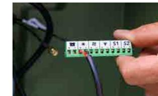
Connect the cables to the inputs + and - in the terminal on the Solar Panels inputs. When the cables are connected, push the terminal back into the FeedCon.
