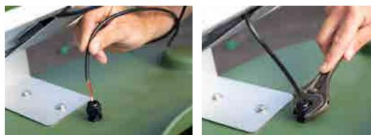
*Note! Tighten the cable glands after the cable is in place.*
